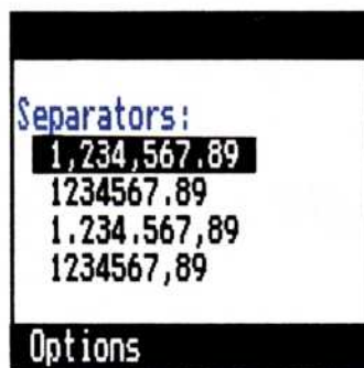
Figure 7-20. The separators option lets you display commas or periods (1) between thousands, hundred thousands, millions, etc., for large values, and (2) at the beginning of the decimal portion of a value.
