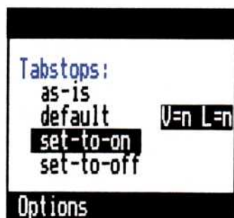
Figure 3-5. You can elect to have cells automatically become tab cells with the "set-to-on" option or turn off this automatic setting by selecting "set-to-off."
