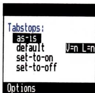
Figure 7-14. The tabstops option lets you set tabs in cells so you can move quickly from cell to cell.
