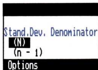
Figure 3-17. You can elect to calculate the standard deviation, treating the list as either the entire value population (N) or as a small sample from some larger population (n-1).
